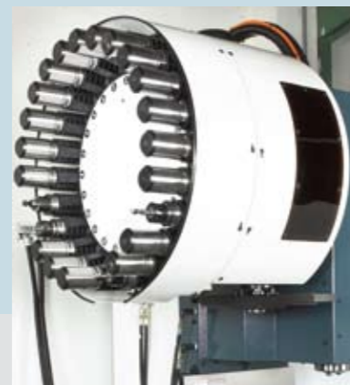
BT30 Arm Type Magazine 20 Tools: Tool to Tool 1.5 sec.
