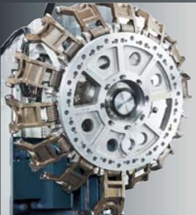
Armless-Type Magazine Tool change time: 1.8 sec. 12 and 14 tools are available
